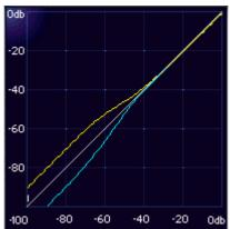
Upper line shows Low-level compression (upward), achieved when Range is negative and Gain is equal but positive. Lower line shows Low-level expansion (downward), achieved when Range is positive and Gain is equal but negative. Graph is taken from C1 to help visualize the gain structures in the LinMB.
